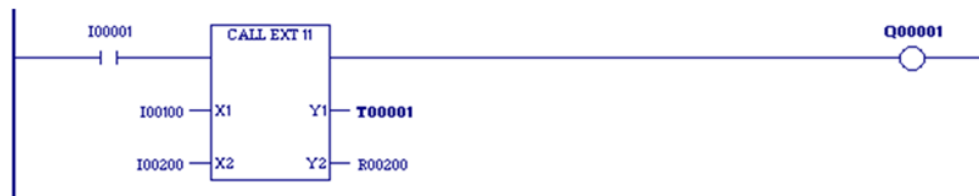
Figure 8: Calling an External Block in Ladder Logic
